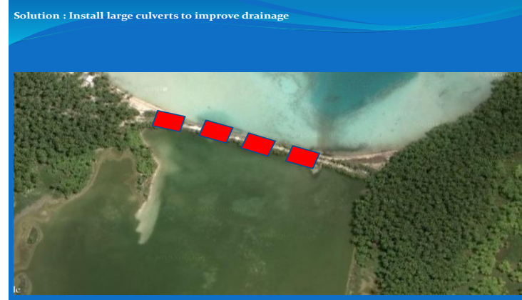
Solution : Install large culverts to improve drainage Red boxes indicate where the culverts will be placed at the mouth of the pond on Rakahanga.
